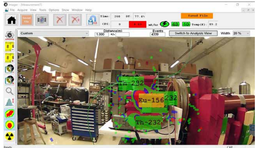
Analysis of the positron accelerator secondary yield with the GeI germanium detector of the Detector Laboratory. Credit: M. Kallikoski.
